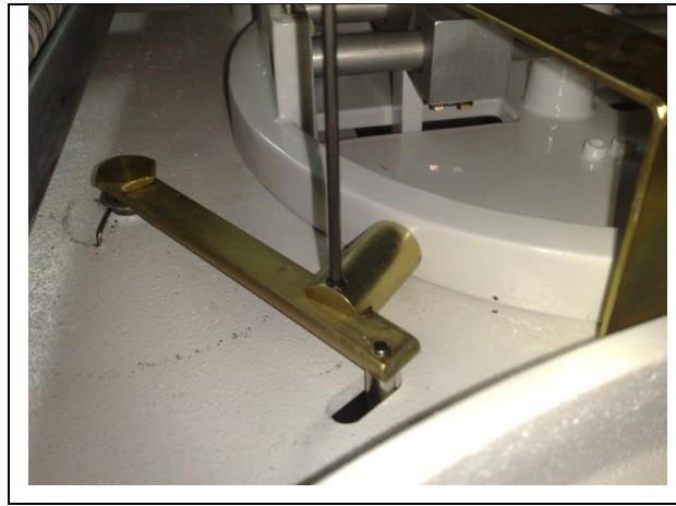
Figure 84 – Rotation adjustment of the ear rods' support
