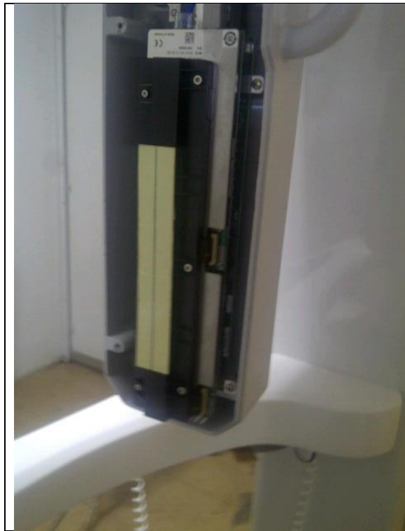
Figure 68. Fluorescent tool in Snap-On Ceph Position.
