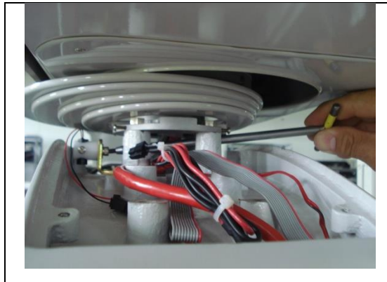
Figure 60. Mid-Sagittal Laser Beam Adjustment Screw.
