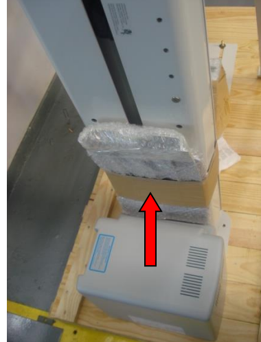
Remove the plastic protection and the rotation arm's plastic cover (f)
