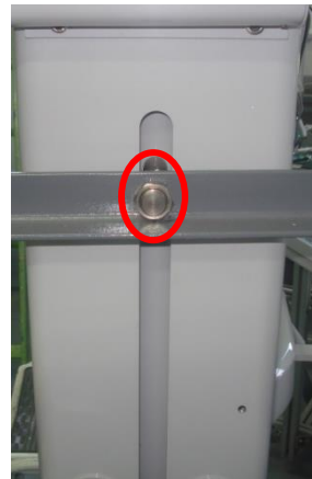
Remove the metallic support by removing the nut in the back of the equipment (h)
