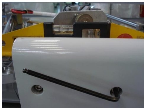
Fix the ceph arm in the ceph head with two screws (i)
