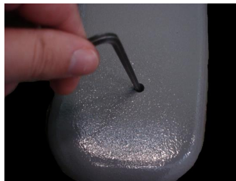
Adjustment of the leveling screws
