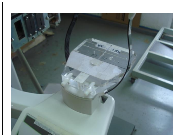
Figure 41 - Pins Phantom above the chin support
