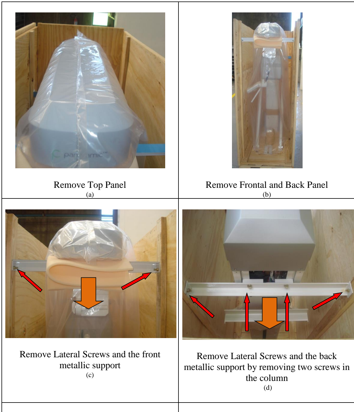
Figure 3. Unpacking the panoramic unit.
