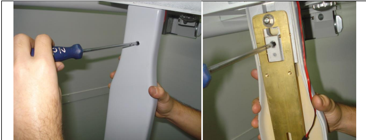
Figure 63. Secondary Collimator Cover Screws
