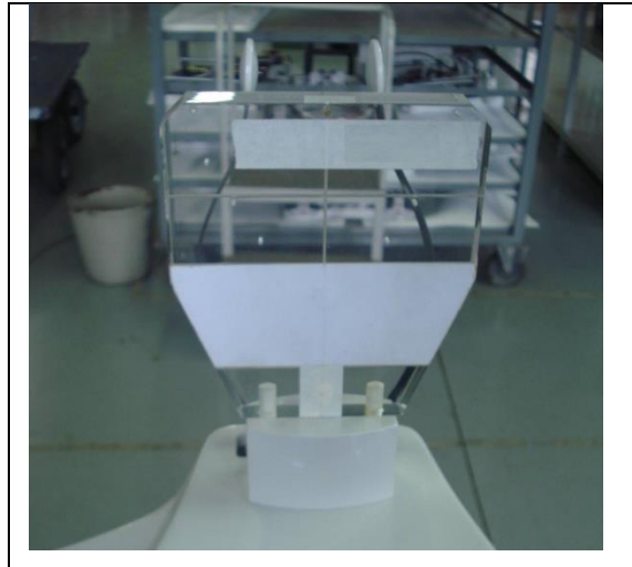
Figure 55 - Phantom in Position for parallelism adjustment of laser beam Frankfurt/Canine.
