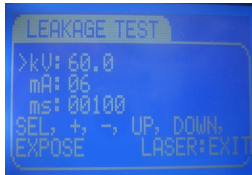
Figure 98 - Leakage test menu
