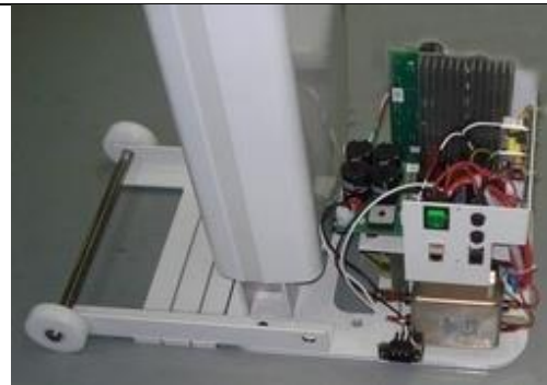
Remove the metallic support by removing the nut in the back of the equipment (h)
