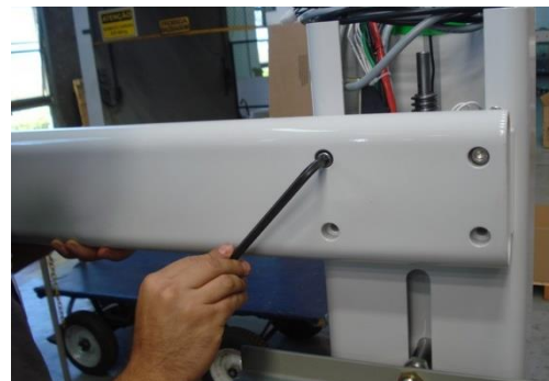
With both systems mount together, fix the ceph system in the panoramic equipment. (j)
