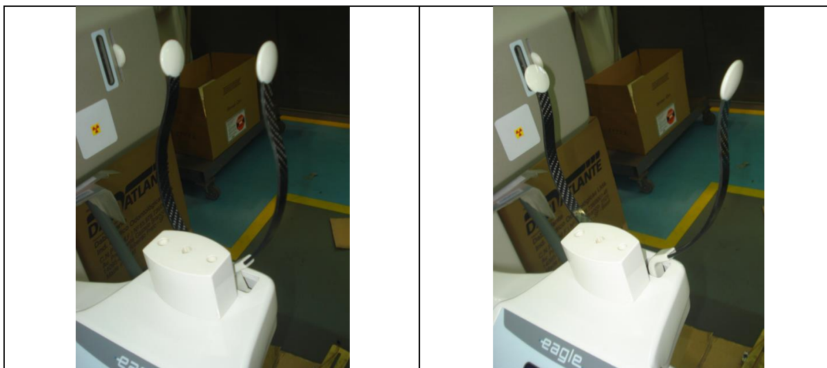
Figure 65 - Opening and locking the head support
