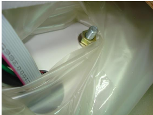
The ceph arm is fixed for two bolts. Remove the nuts and bolts. (g)
