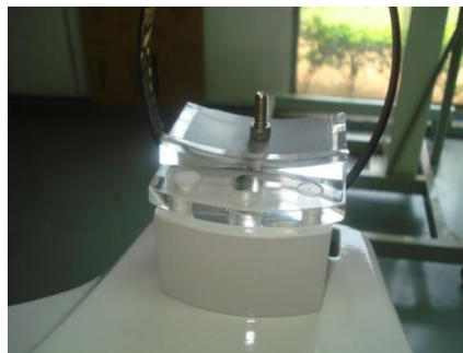
Figure 37 - Screw above the chin support
